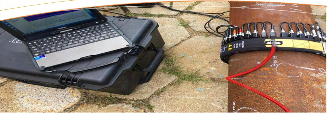
LRUT is used to detect corrosion, erosion in pipe work. An array of transducers is clamped around the pipe and ultrasound is transmitted simultaneously along the pipe in both directions. The return signal is received by the same transducers, and the data are analyzed using the system's calibrated software.
